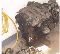
The pictures above show a typical 6A. This is pretty much the state that mine arrived in although I have already taken the water pump off in these pictures. Things to notice are the position of the throttle body on the top of the inlet manifold, the shape of the sump, the oil cooler and the crank case breather. I'll return to each of these issues as we go along.
